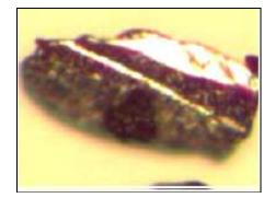
**Figure 6: Fatigue Wear Particles**
