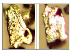
Figure 5: Fatigue Wear Particles of Straight Edges
